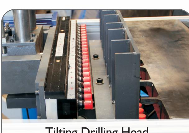
Tilting Drilling Head Can do accurate hole on surface
