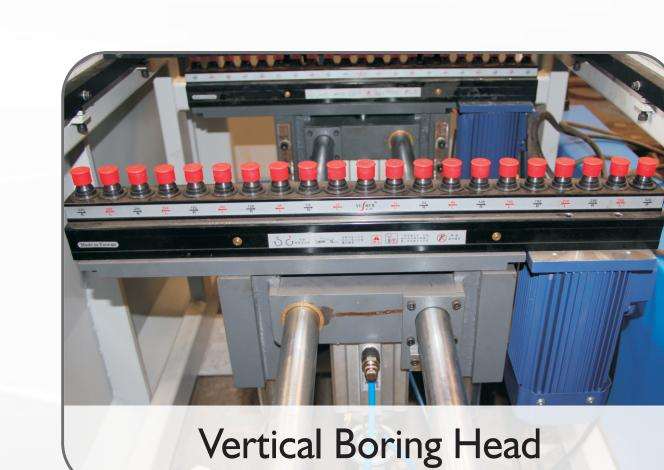
• 21 drilling bits at 32mm distance.
