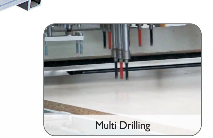
Five horizontal and five vertical drilling bits.
